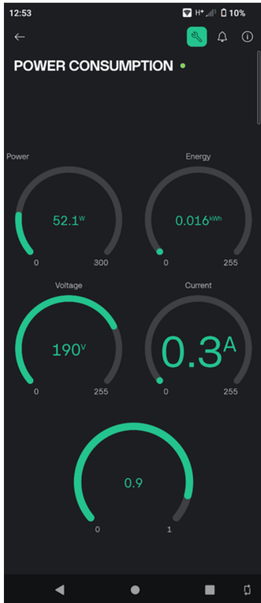
Figure 9. Blynk widget monitoring of energy usage on smart phone
