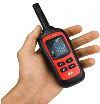
Figure 3.2. Digital thermo-hygrometer used for measuring air temperature and relative humidity
