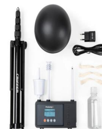
Figure 3.4. Thermal comfort measurement kit including a black globe thermometer
