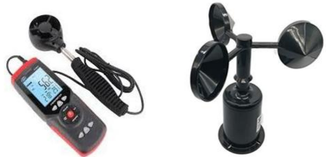
Figure 3.3. Anemometers used for measuring air velocity
