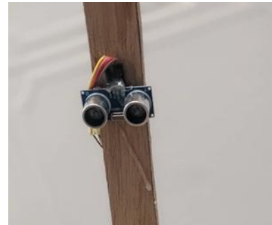
Fig. 5. Ultrasonic sensor mounted on the frame for height sensing.
