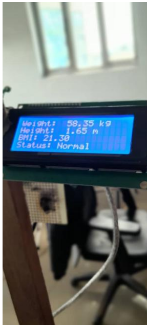
Fig. 7. Prototype display showing weight, height, BMI and a Normal-weight status.
