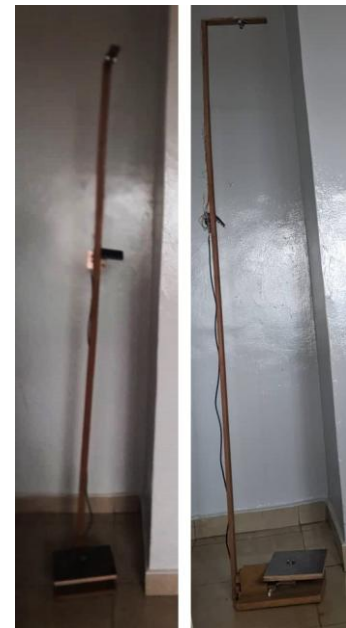
Fig. 6. The assembled BMI monitoring prototype (front and side views).
