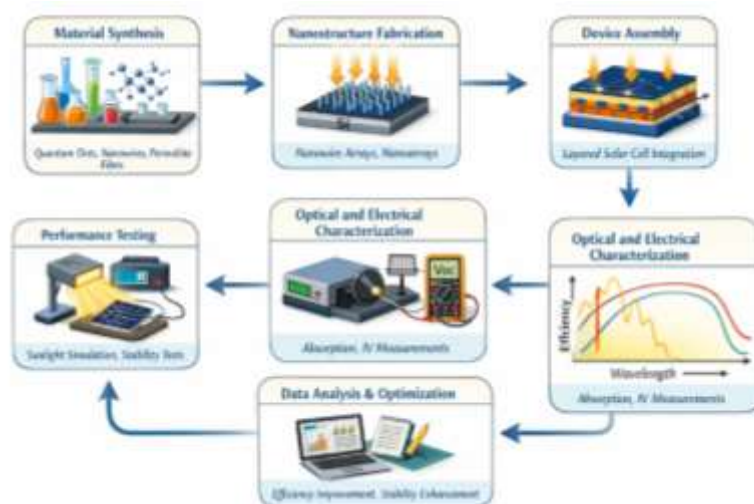
Figure 3. Procedures for enhancing work solar cell using Nanotechnology.
