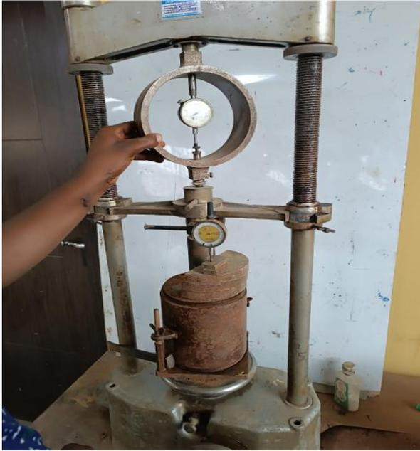
Fig. 5: CBR test machine used in CBR test determination.
