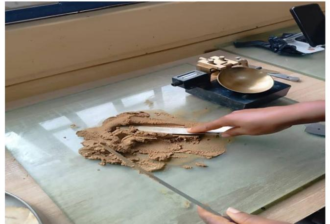
Figure 2: Casagrande apparatus setup for Atterberg limit testing, showing the liquid limit determination
