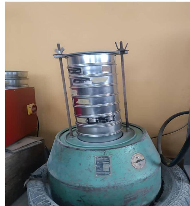
Fig.2: Set British Standard sieves on shaker
