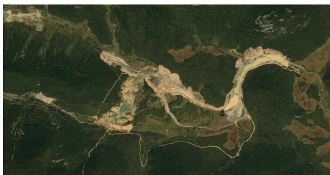
Fig. 1. Dump complex formed as a result of the development of the Maly Algiyak placer deposit.
