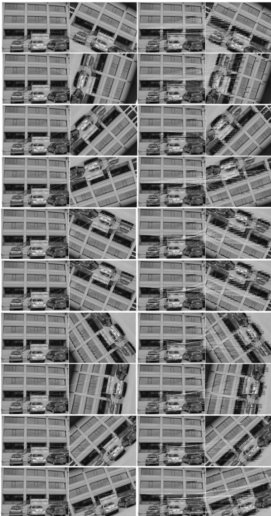
Fig. 9. Harris (Left Images) vs SIFT (Right Images) Rotating Results
