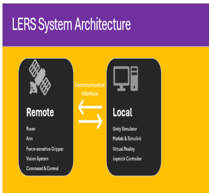
Fig. 2. LERS High-Level System Architecture
