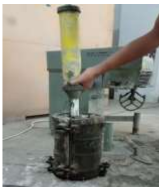
Fig. 3. Grouting Pumping Process
