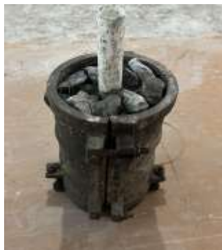
Fig. 2. Placing Coarse Aggregate and Rebar Wire Fiber in the Cylindrical
