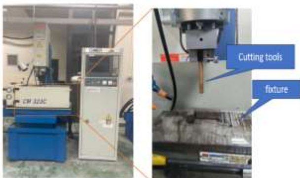
Fig. 1. Image of experimental equipment and copper electrode for electric spark pulse machining
