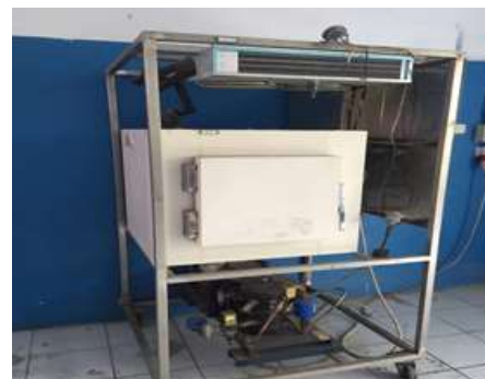
Fig. 1. TD242 Refrigeration system
