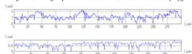
Fig. 12. Machined Surface Profiles with SD 400# and SD1500# Wheels Obtained by Mitaka
