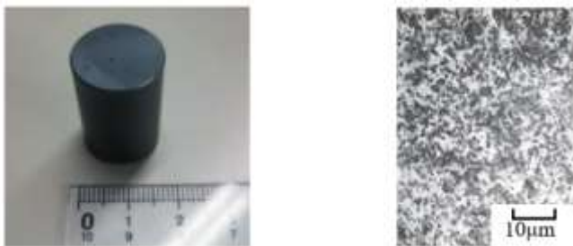
Fig. 2. CVD-SiC workpiece and Micrograph of Surface
