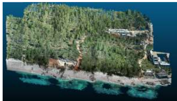
Fig. 5. Point Cloud generated from Aerial Photogrammetry using Pix4Dmapper.
