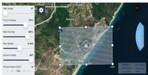
Fig. 2. UAV LIDAR flight mission planning with DJI Matrice 300 RTK L1.
