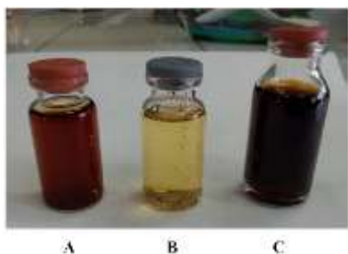
Fig. 3. Liquid smoke in conditions (A) before distillation, (B) distillation results, (C) undistilled part
