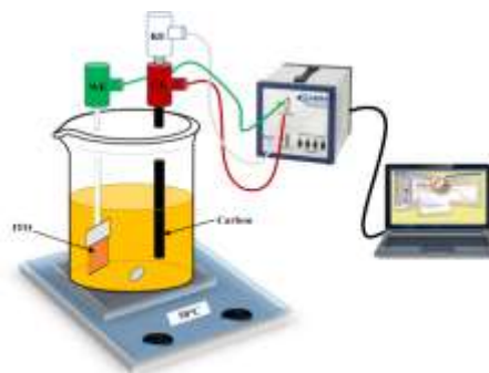
Fig. 3. Electrochemical deposition system with two electrodes
