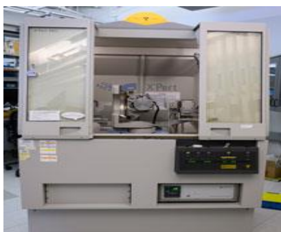
Fig. 2. (XRD) Measurement unit utilized.
