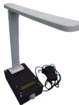
Figure 2. Automatic Lighting System in Library Reading Room
