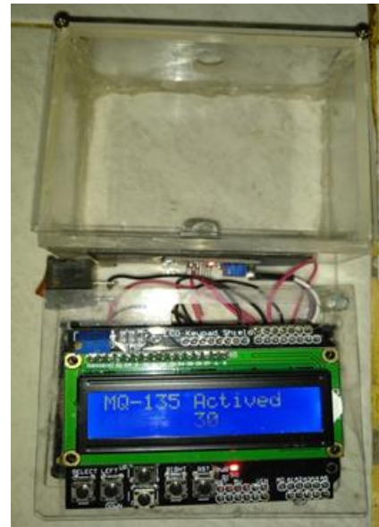
Figure 3. Detection of ammonia content
