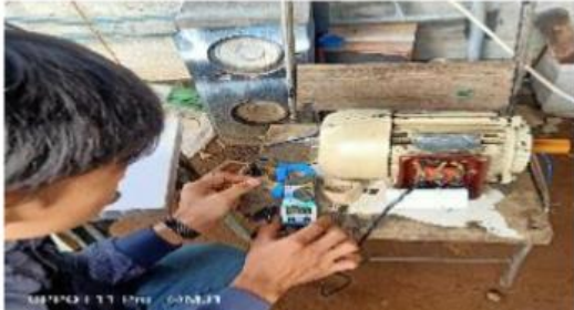
Figure 3. Three Phase Motor Measurement No Load
