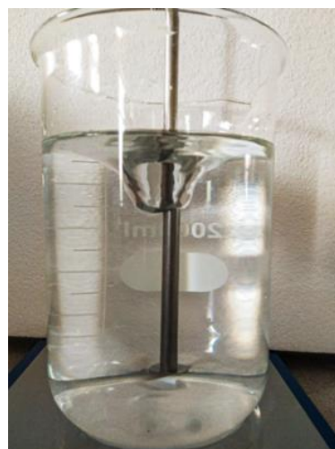
Fig. 6. Vortex formation with pitched blade stirrer
