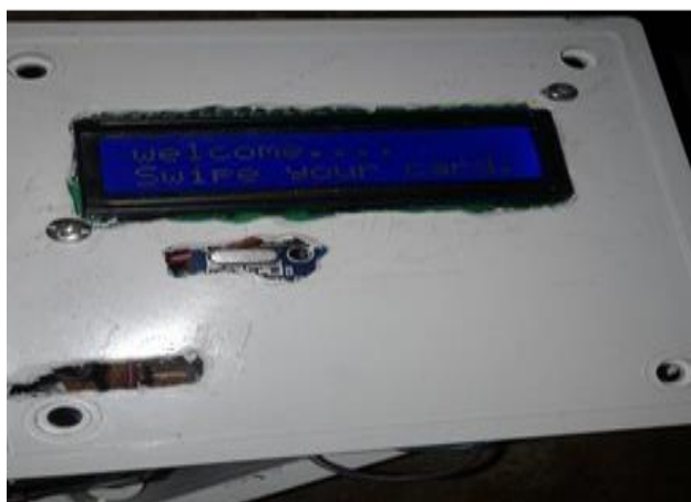
Fig. 5. System is ready to read the RFID card
