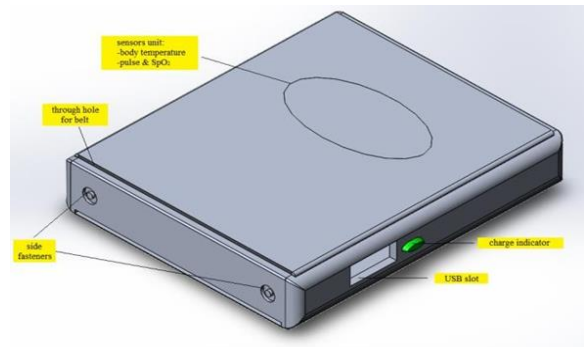
Fig. 4. The case of the device. Bottom view
