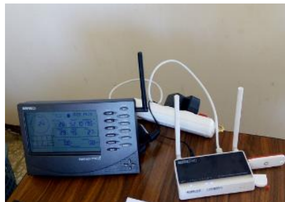
Figure 5: Implemented Wireless Weather Station
