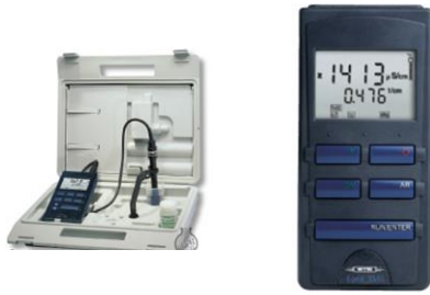
Figure 8: Implemented Salinity measuring device
