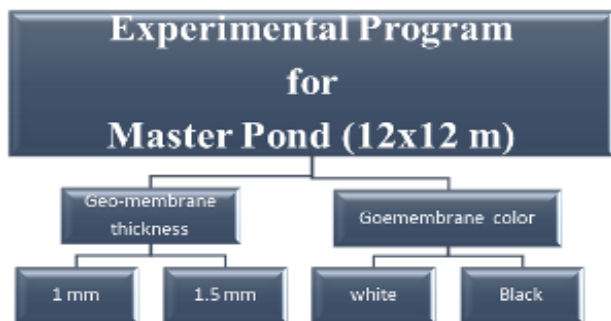
Figure 2: Experimental Program for the different parameters
