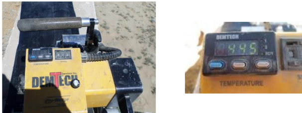
Figure 16: Implemented wedge welder and temperature
