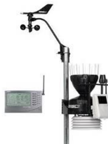
Figure 7: Implemented Wireless Weather Station after assembly
