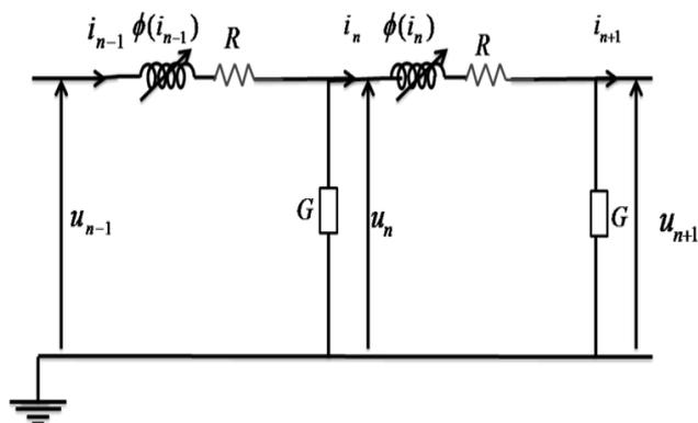
Fig. 1. Presentation of a nonlinear inductive electrical line.
