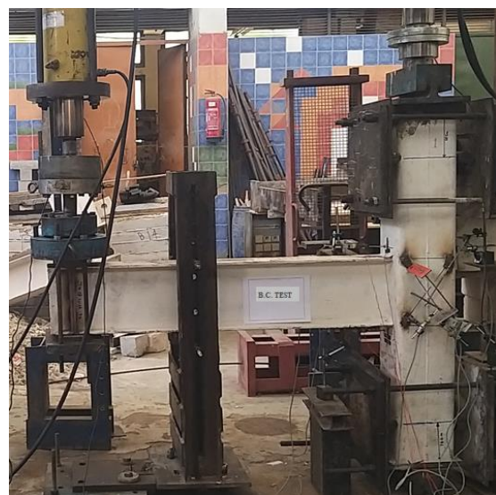
Fig. 2. Test setup and Loading system (All Dim. in mm)
