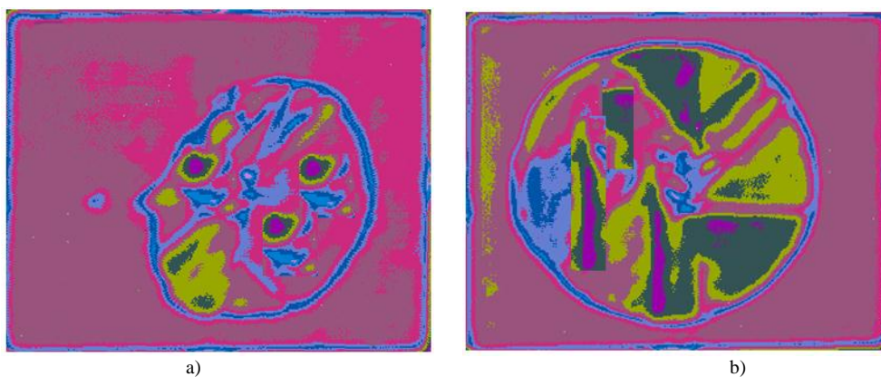
Fig. 11. C-scan image of 30J and 50J impacts using the flat impactor [1], [10].
