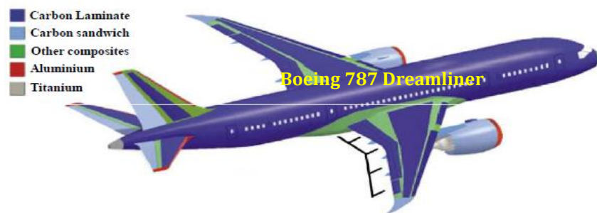
Figure 1: Breakdown of materials used in the Boeing 787 Dream liner [1]
