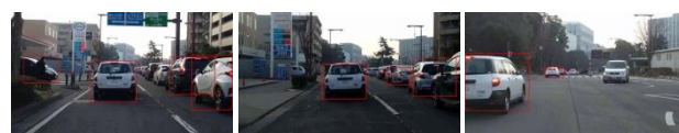
The detection results of the 1794,1859 and 2129 frames from video based on SSD model
