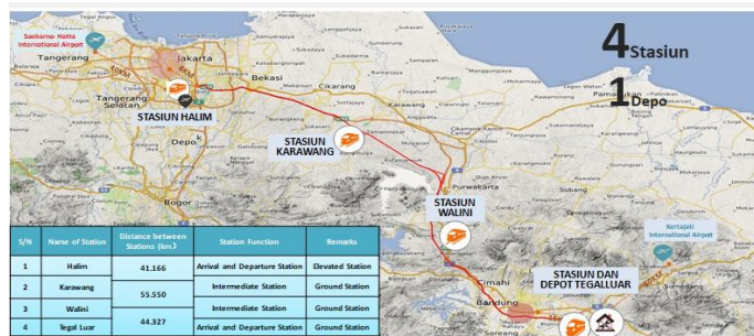
Fig. 2. Alignment and Station & Depot Location Train of HSR Jakarta – Bandung Project
