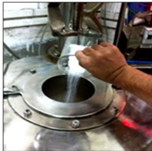
Figure 5: Addition of nano particles in melting and blending unit with nylon-jute fibre paste
