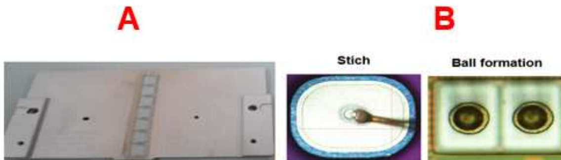
Fig. 3. a) Enhanced process plate design, b) Actual stitch and ball formation improvement.
