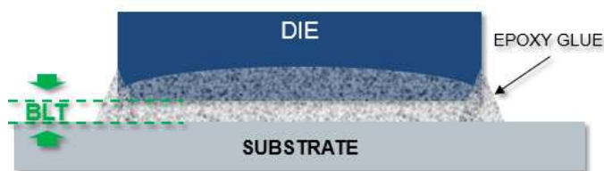
Fig. 1. Package cross-section showing BLT.
