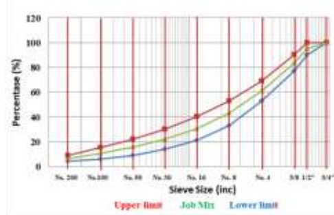
Fig. 1. AC-WC Aggregate copimnent Sieve Analysis
