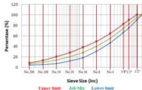
Fig. 2. AC-BC Aggregate copimnent Sieve Analysis
