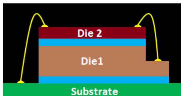
Fig. 2. Stacked dice configuration.
