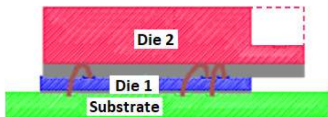
Fig. 3. Device A package cross-section view.
