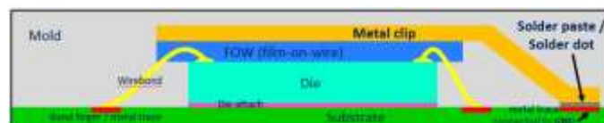
Fig. 2. 2D illustration of an IC with metal cover design.
