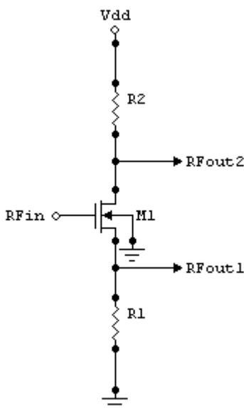
Fig. 1. Schematic diagram of common-source/drain active balun.
