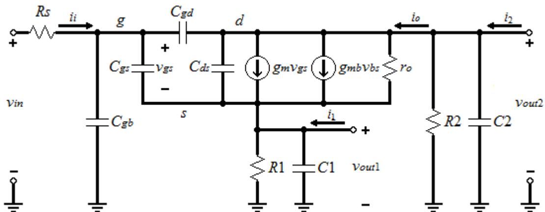
Fig. 2. Common-source/drain active balun high frequency small-signal circuit.
