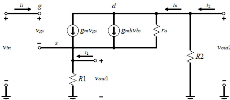
Fig. 3. Common-source/drain active balun low frequency small-signal circuit.
