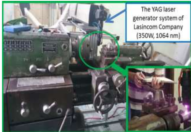
Fig. 1. Experimental design of the laser-assisted turning 9CrSi hardened steel.
