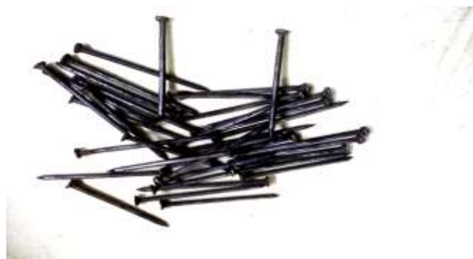
Figure 6. Rusty nails boiled with cassava wastewater
