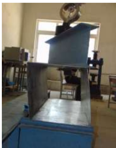
Fig. 2 (iii) Failure mode shape of Box section
