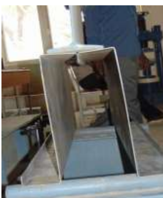
Fig. 4 (iii) Failure mode shape of Z-section
