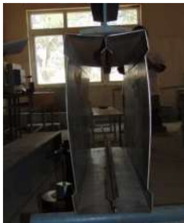
Fig. 6 (iii) Failure mode shape of sigma section
