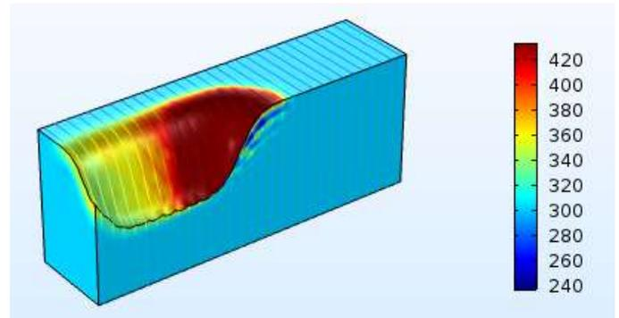
Fig. 3. 3D view of temperature distribution in workpiece at laser cutting speed of 4m/min.
