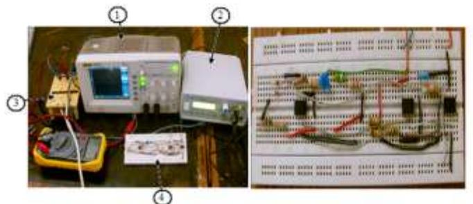
Fig. 2. left: Photograph of the experimental circuit consisting of: (1) An oscilloscope necessary to visualize signals, (2) The low frequency signal generator used to force the oscillator, (3) A source of operational amplifiers polarizations, and (4) the corresponding oscillator's circuit depicted in Fig.1, which is zoomed in the right.
