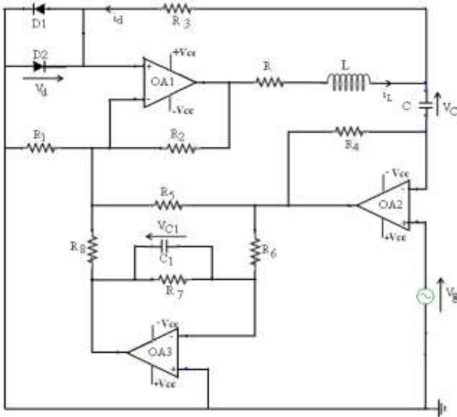
Fig. 1. Circuit diagram of the Duffing-Holmes chaotic pulse oscillator, driven by the low frequency signal generator  $V_g$ .
