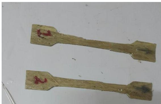
Fig. 7. Tensile strength specimens.
