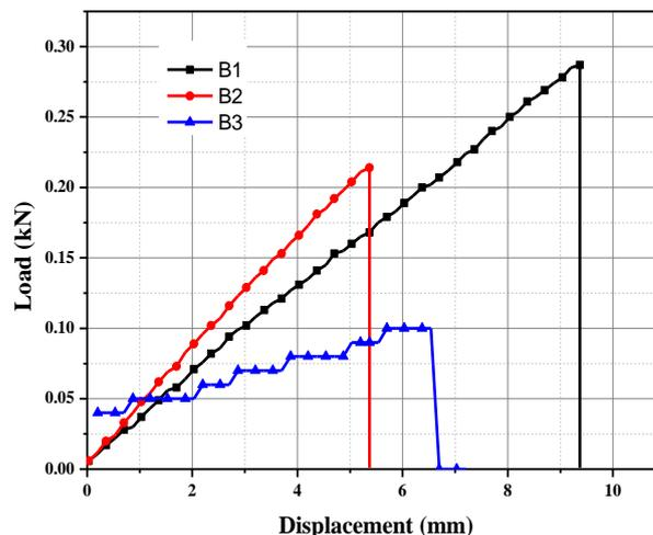
Fig. 12. Load-displacement curve of three point bending test.
