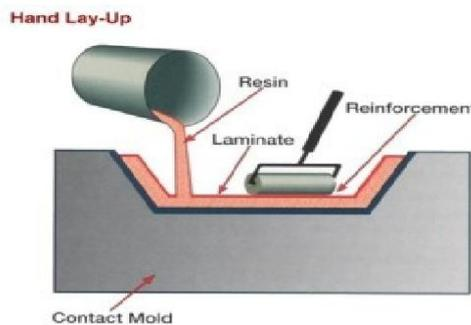
Fig. 3. Hand lay-up molding.
