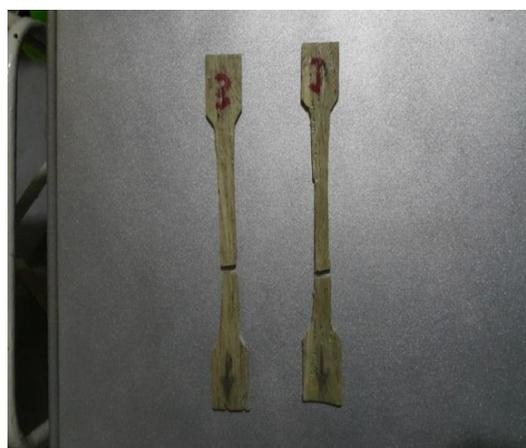
Fig. 9. Failure of tensile test.
