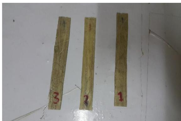
Fig. 8. 3-point bending specimens.
