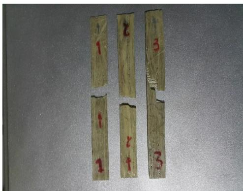
Fig. 11. Failure in bending test.
