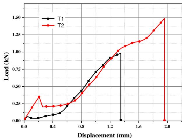
Fig. 10. Load- displacement curve of tensile test for banana fiber reinforced composite.
