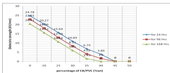
Fig. 3. Dielectric breakdown strength of CB/ PVC composites at 70°C for 24, 96 and 168Hrs under thermal aging.
