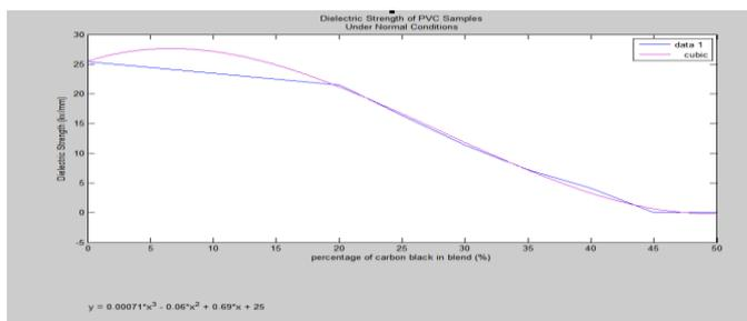
Fig. 7. Curve fitting of dielectric strength for PVC samples loaded with carbon black filler with various percentages under normal condition.
