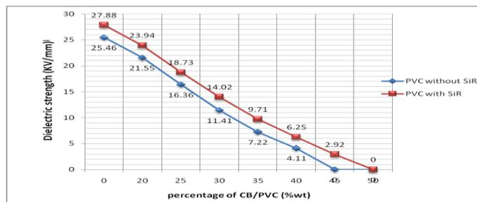
Fig. 2. The dielectric breakdown strength of CB/PVC composites with and without SiR under normal conditions.
