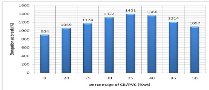
Fig. 6. The elongation at break for PVC samples loaded with carbon black filler with various percentages under normal condition.
