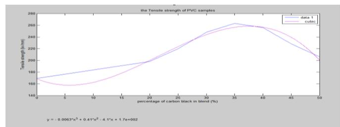
Fig. 15. Curve fitting of tensile strength for PVC samples loaded with carbon black filler with various percentages under normal condition.
