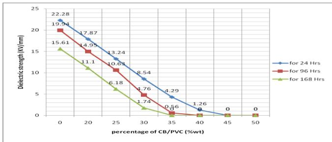
Fig. 4. Dielectric breakdown strength of CB/ PVC composites at 90°C for 24, 96 and 168Hrs under thermal aging.
