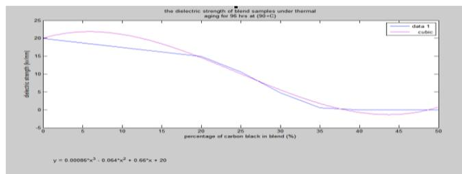
Fig. 13. Curve fitting for the dielectric strength of PVC samples loaded with different carbon black filler percentages under thermal Aging for 96 hrs at (90°C).
