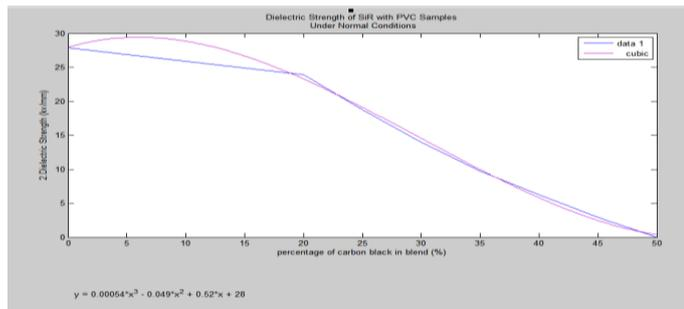
Fig. 8. Curve fitting for the dielectric strength of PVC Samples with different carbon black filler percentages with SiR layer under normal condition.
