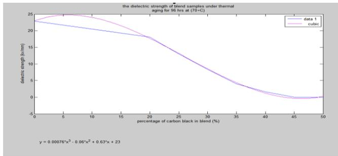
Fig. 10. Curve fitting for the dielectric strength of PVC samples loaded with different carbon black filler percentages under thermal Aging for 96 hrs at (70°C).
