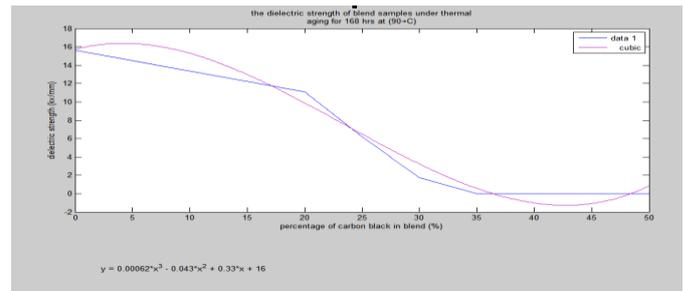
Fig. 14. Curve fitting for the dielectric strength of PVC samples loaded with different carbon black filler percentages under thermal Aging for 168 hrs at (90°C).
