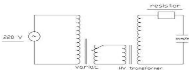
Fig. 1. Schematic diagram for the dielectric strength testing circuit.
