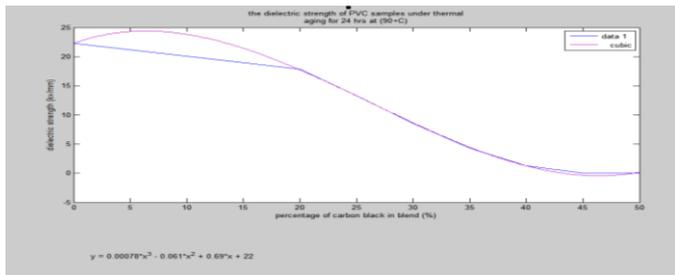
Fig. 12. Curve fitting for the dielectric strength of PVC samples loaded with different carbon black filler percentages under thermal Aging for 24 hrs at (90°C).
