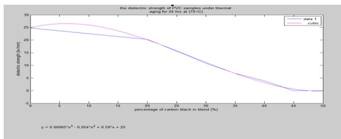
Fig. 9. Curve fitting for the dielectric strength of PVC samples loaded with different carbon black filler percentages under thermal Aging for 24 hrs at (70°C).
