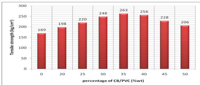
Fig. 5. The tensile strength of CB/PVC composites under normal conditions.
