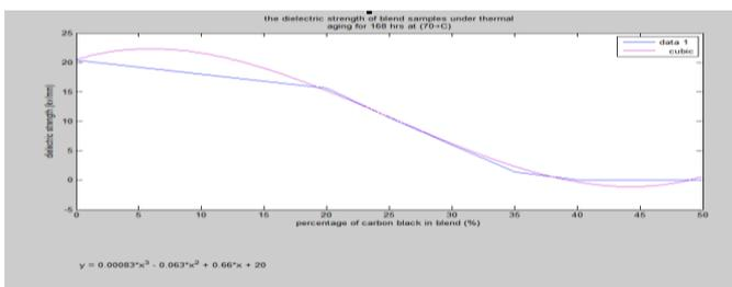
Fig. 11. Curve fitting for the dielectric strength of PVC samples loaded with different carbon black filler percentages under thermal Aging for 168 hrs at (70°C).
