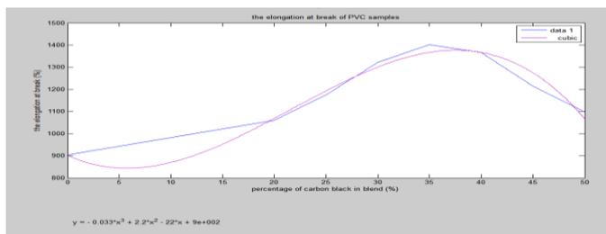
Fig. 16. Curve fitting of elongation at break for PVC samples loaded with carbon black filler with various percentages under normal condition.
