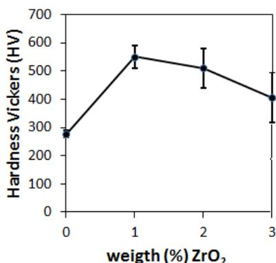
Fig. 6. The effect addition of zirconia to the hardness of barium ferrite. The zirconia has given strengthening to barium ferrite as ceramic matrix composite.
