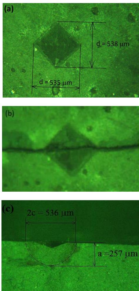
Fig. 2. (a) Vickers Indentation to determine initial crack on the B3B-K<sub>1c</sub> methode, (b) the fracture of the specimen after B3B biaxial testing (c) The surface crack by Vickers indentation in form a semi-circular to determine 2c and a, from cross section side.
