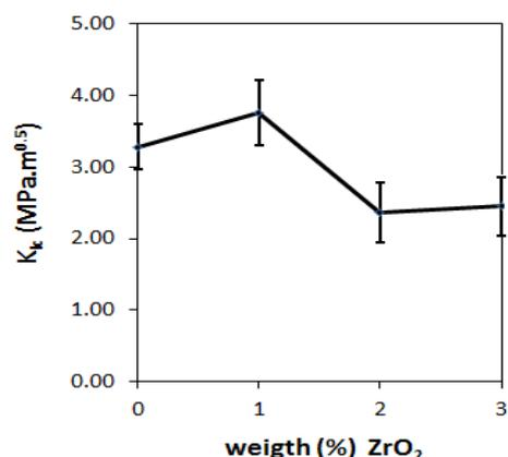
Fig. 8. The effect of zirconia to the K<sub>IC</sub> of the barium ferrite.
