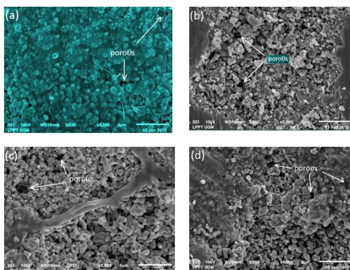
Fig. 4. SEM Photograph of barium ferrite phase with the various addition of zirconia by weight %, (a). barium ferrite phase, (b). 1% ZrO<sub>2</sub>, (c). 2% ZrO<sub>2</sub>, (d). 3% ZrO<sub>2</sub>.
