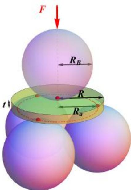
Fig. 1. The B3B testing methods with a disc-shaped test specimen with a radius  $R$  and the thickness  $t$ ,  $R_a$  support radius (distance between the center of the load to the supporting balls). Force  $F$  is applied through the ball parallel to the centre axis of the disc [5].
