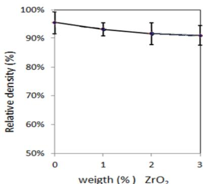
Fig. 5. The relative density barium ferrite with various weight % zirconia was tested by using Archimedes method.
