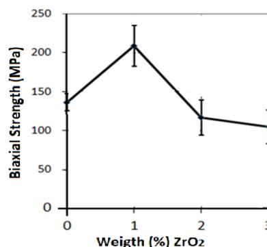
Fig. 7. The effect of zirconia to the biaxial strength of barium ferrite.
