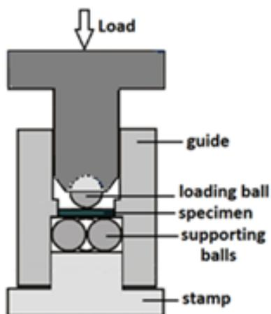
Fig. 3. Schematic of test equipment biaxial strength by the B3B method
