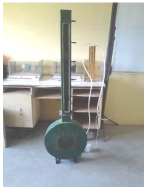
Plate 1. Set up apparatus for terminal velocity measurement.
