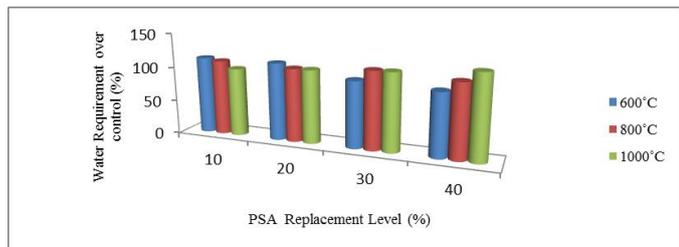
Fig. 3. Water Requirement of Periwinkle Shell Ash Calcined at Different Temperatures for Mix Ratio of 1:1:2.
