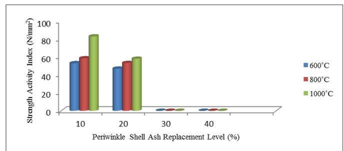
Fig. 2. 28 Days Compressive Strength Activity Index for Mixed Ratio of 1:2:4.
