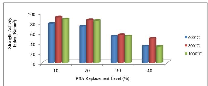
Fig. 1. 28 Days Compressive Strength Activity Index for a Mixing Ratio of 1:1:2.
