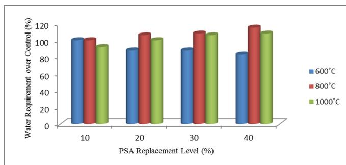
Fig. 4. Water Requirement of Periwinkle Shell Ash Calcined at Different Temperatures for Mix Ratio of 1:2:4.
