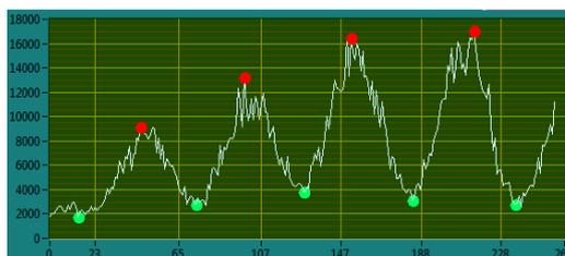
Fig. 11. The compressed 1D noisy interferogram with unique peak and valley identification.
