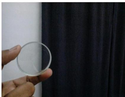
Fig. 1. Sample phase plate (two sprayed glasses sandwiched).
