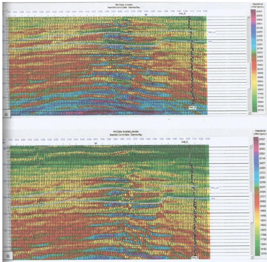
Fig. 2. Inverted Seismic section of (a) Base and (b) Monitor with PH2\_v2 and PH2 Horizons.
