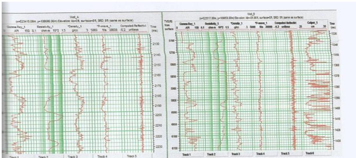
Fig. 3. Suite of raw well logs A & B before applying median filter to P-wave and density logs and also check-shot correction.
