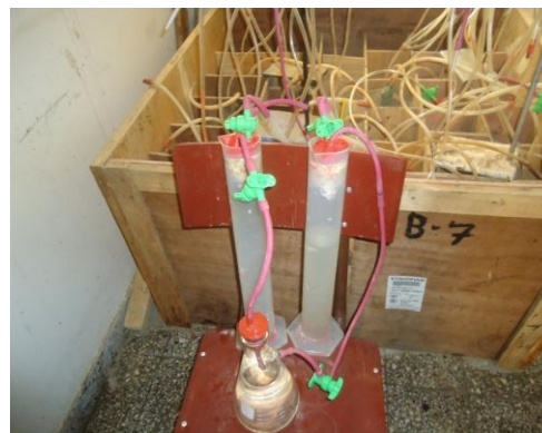
Figure 3.1 Set up of the experiment of biogas production and the residue of the feedstock used as bio-fertilizer.
