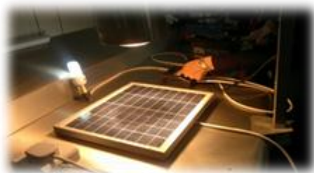
Fig. 2. Solar simulator used in the tests
